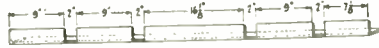
FIG. 13 By marking the brass angle according to the dimensions given above, sawing out the undesired portions, and then bending the brass to shape, a firm support for the aluminum bed-plate is obtained.
