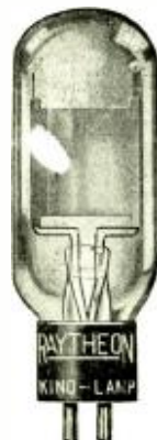
A form of conductive-gas lamp. It is similar to the neon-filled lamps, in operation. The square surface becomes intermittently luminous so rapidly the eye cannot possibly follow the fluctuations. It is this "optic fatigue" which makes television possible.
